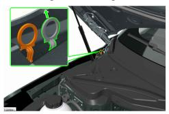
3. Pull the white ring and unlock the charge cable and reposition the ring to its original position.
