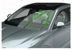
3. Press the wiper blade locking button (A) and remove the wiper blade (B).
