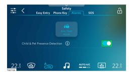
• Tap on the child & pet presence detection button to activate or deactivate the function.
