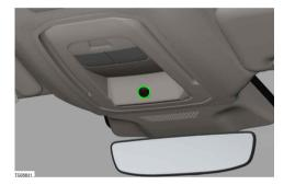
The in cabin camera is mounted on the overhead console. Using the Trumore app, occupants can capture both pictures and videos.
