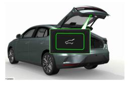
Press the tailgate inside switch to close the tailgate.
