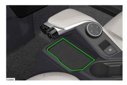
You can charge your mobile phone wirelessly using the wireless charging mat at the center console.
