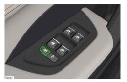
Press the button to lock or unlock the rear window control for passengers.
