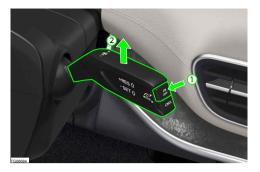
If adaptive cruise control is set at the desired speed and then the brakes are applied or button (1) is pressed, the cruise control is deactivated without erasing the set speed from memory.
