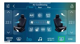
Tap on the rear window heating button to activate/ deactivate the rear window heating.
