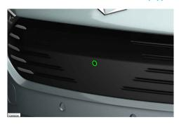
For vehicles equipped with the surround view feature, a camera is provided on the shield assembly. It is used to provide visual information when parking and maneuvering the vehicle.
