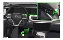
To cancel the adaptive cruise control, press the button (1) or press the brake pedal (2).
