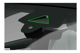
The front smart camera is located behind the windshield. The front smart camera provides information to various driver assistance features.
