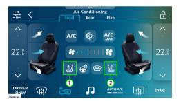
Tap on the (1) or (2) seat heating button to adjust the heating level of the driver or front passenger seat.
