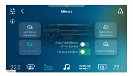
Tap on the parking position button to activate/ deactivate the function.
