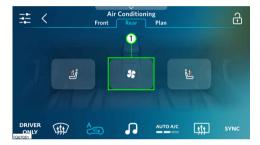
Tap the button (1) on the control display to activate/deactivate the blower for rear row.
