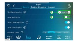
To enable the high beam light assist function, tap on the auto high beam button (2).
