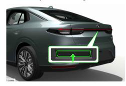
2. Lift the tailgate using the soft touch handle to open it.
