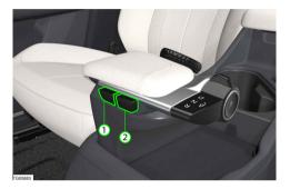
Select the desired level of recuperation or deactivate the recuperation function using the gear shift unit buttons (1) or (2).
