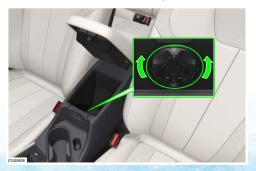
Rotate the vent wheel counterclockwise or clockwise to turn On/Off the cooling.
