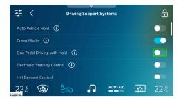
Tap on the one pedal drive with hold button to activate or deactivate the one pedal drive with hold function.
