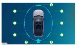
The 360° view displays the vehicle surrounding along the front, rear, and sides of the vehicle, when active. Different views of the vehicle can be displayed by touching at different camera angles (1). The camera view icon (2) is displayed on the selected view and an image is displayed on the main screen.
