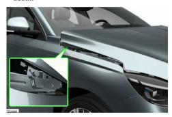
The active hood is designed to enhance pedestrian safety by reducing the risk of injury in the event of a front-end collision. When a collision occurs at speeds between approximately 25 - 55 km/h, sensors located in the frontal area detect the impact and trigger the system. This action raises the rear portion of the hood by several centimeters, creating an additional crumple zone to help protect a pedestrian's head.
