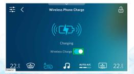
Tap on the wireless charge button to activate/ deactivate the function.
