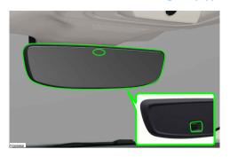
The rearview mirror is dimmed automatically depending upon the brightness measured by two light sensors.
