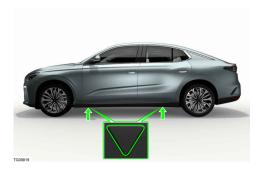
The reinforced jack attachment/lifting points are available on the area behind the triangles on the rocker molding.
