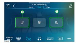
• Tap on the (1) or (2) seat heating button to adjust the heating level of the left or right seat.
