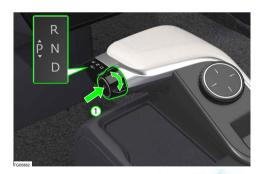
Use the gear selector to switch the drive position. The brake pedal must be pressed while engaging the drive position from "P". When the vehicle is ready to drive, the drive modes and selected gear are displayed on the driver's screen. (Refer to 6.2.1.3 Center tile)
