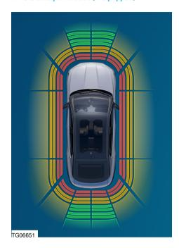
The side park assist function warns you of any obstacles detected to the side. The obstacles must be detected in advance by the front or rear ultrasonic sensors while driving by them. If the vehicle is steered in the direction of a detected obstacle and a lateral collision is imminent, an audio and visual warning is issued.
