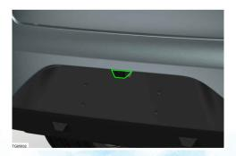
The rearview camera is located on the rear bumper. It is used to provide information when parking and maneuvering the vehicle in reverse.
