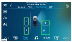
4. The auto park in completion is indicated on the main screen. If required, adjust the parking position and select the shift lever to "P" mode.
