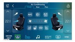
Tap on the max defrost button to activate/ deactivate the max defrost.
