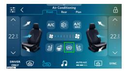
Tap on the windshield heater button to activate or deactivate the windshield heater.
