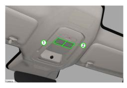
Switching front reading light On/Off
