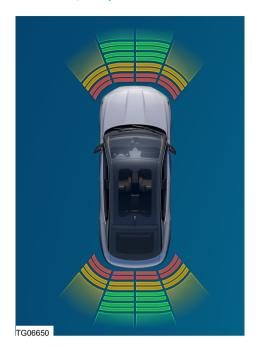
When the front assist function is activated and vehicle speed is below 15 km/h, the ultrasonic sensors will detect the proximity of an obstacle from the front or rear bumper and this information is displayed on the main screen and driver's screen.
