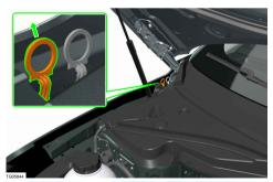
3. Pull the orange ring and unlock the charging lid and reposition the ring to its original position.
