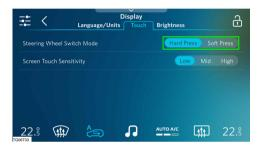
Tap on the button to set the desired steering wheel switch mode.
