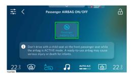
• Tap on the button to activate or deactivate the passenger airbag.
