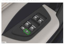
Use the lock button (1) on the driver's door to lock or unlock all the doors and the tailgate at the same time.
