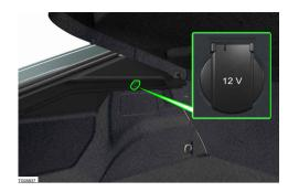
The 12V power outlet in the trunk compartment can be used to connect the electrical accessories. The power usage from the sockets must not exceed a total of 120 watts. Do not connect multiple devices to the sockets in the vehicle at the same time. The 12V power outlet is labeled with the 12V symbol.
