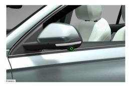
For vehicles equipped with the surround view feature, a camera is provided on both outside mirrors.
