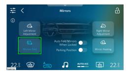
Tap on the mirrors fold button to fold the outside mirrors.
