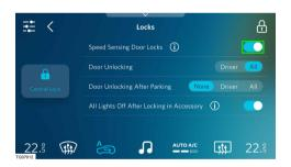
Tap on the speed sensing door locks button to activate/deactivate the speed sensing door locks function.
