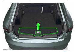
The tire repair kit is located in the trunk storage box.
