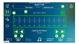
You can receive available radio stations on different frequency bands and store your favorites to station for main controls. The radio supports the FM and DAB (Digital Audio Broadcasting) frequency ranges.
