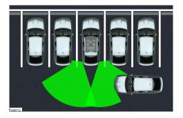
The rear cross traffic alert system can help alert the driver of an approaching vehicle or objects behind the vehicle while the vehicle is reversing, for example, pulling out of a parking space.
