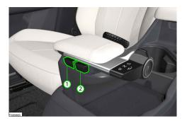
2. Select the desired drive mode using the control display or GSU buttons (1) or (2).
