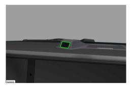
The driver infrared camera monitors the alertness and condition of the driver. It can detect distraction, drowsiness, and microsleeps and can alert the driver in time. For more information on driver monitoring system, Refer to 4.8.1.3 Driver Monitoring System.
