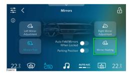
Tap on the mirror heating button to activate/ deactivate the outside mirror heating.
