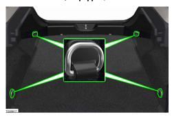
There are "4" tie bracket hooks on the side trim panel in the trunk storage compartment to secure pieces of luggage and objects. It can be used in combination with lashing straps, tensioning straps, or retaining straps.
