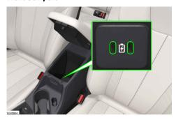
The vehicle is equipped with two USB ports located under the front armrest. Open the jumbo box to access the USB ports. (Refer to 9.4.1 Front Armrest )
