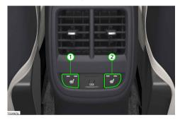
• Press the (1) or (2) seat heating button to adjust the heating level of the left or right seat.
