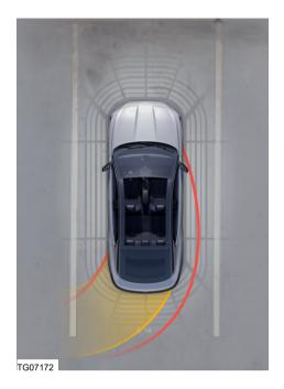
Trajectory lines are displayed behind, in front of or to the sides of the vehicle depending upon the direction of travel. It assists while taking turn or parking the vehicle in tight parking space.
