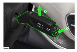
If the intelligent cruise control is set at the desired speed and then the brakes are applied or cancel button (1) is pressed, the intelligent cruise control is disengaged without erasing the set speed from memory.
