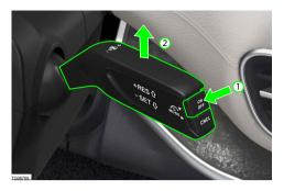
If the speed limit is set at the desired speed and then the button (1) is pressed, the intelligent speed limiter is deactivated without erasing the set speed limit from memory.
