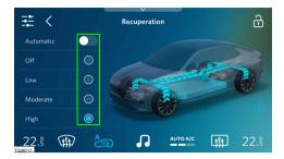
Tap to select the desired level of recuperation or deactivate the recuperation function.
