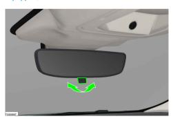
The rearview mirror can be adjusted manually using a lever.
