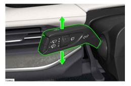
The direction indicators can be activated using the left lever on the steering wheel.
